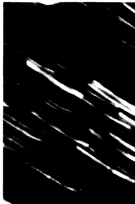
Figure 2. Micrograph of block copolyester VIII between crossed polarizers. 100 \times magnification.
